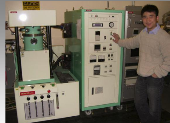
Spark-Plasma Sintering System (MPS) Dr. Sinter 515S at SDSU. Max Load 50kN, max current 1500 A
